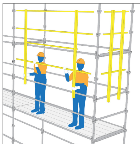
Fig. 3.1.2 Erecting and dismantling temporary scaffolding
