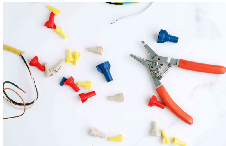
Fig. 4.1.23: Termination of electrical wires/cables by wire nuts
